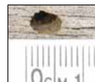
EHB exit hole. – Picture not to scale (CD Pless and G Schweiger UT E&PP)
