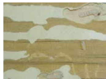
The tunnels created by larvae, as pictured here, can not usually be seen from the surface of the wood – the damage remains hidden
