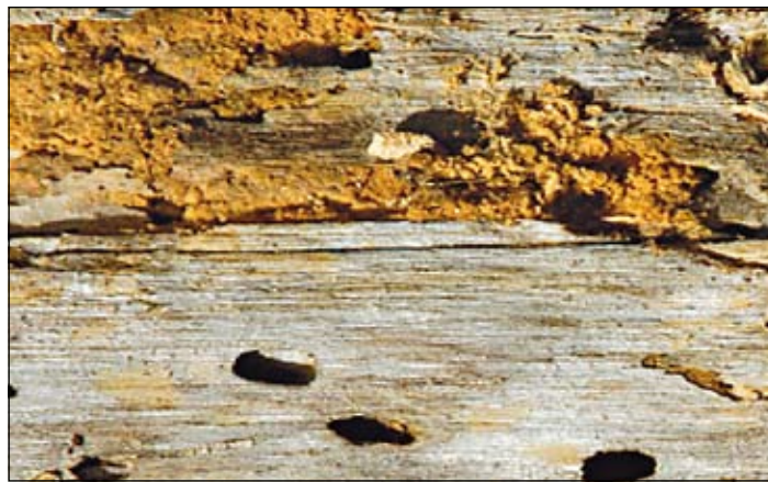
Blisters and emergence holes resulting from EHB infestation
