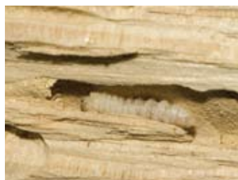
The tunnels created by larvae, as pictured here, can not usually be seen from the surface of the wood – the damage remains hidden
