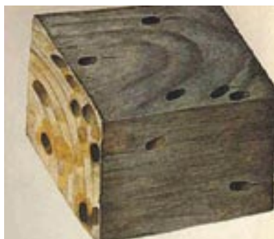
Off-cut of timber exhibiting oval-shaped exit holes caused by emerging adult beetles.
